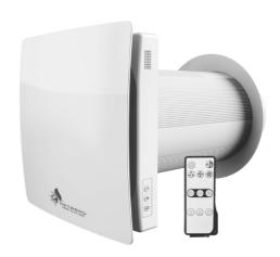
**AT501** systems are direct interface between the inside air and the outside air, installed in a sleeve that passes through the wall. **AT501** systems work in pairs: units are wired together to ensure the house is not pressurized or depressurized, one blows in while the other blows out; then after about a minute, they both reverse directions.
